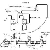
A typical installation injecting chlorine into a pipe line using city water.
