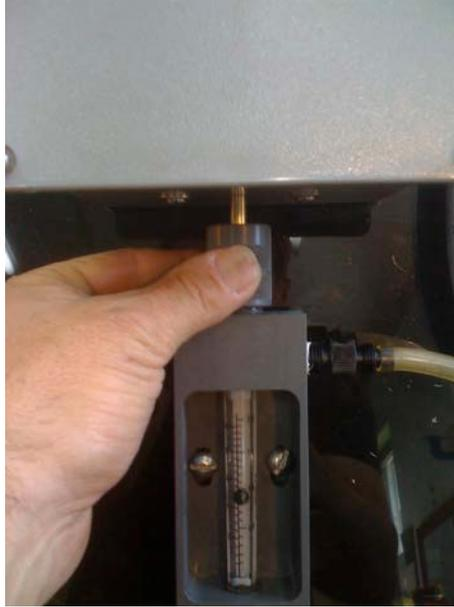
The valve will proportionately adjust the gas feed rate based on the input from the flow meter. Advanced calibration (if needed) is detailed later in the manual.
